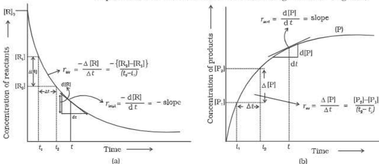
**Fig. 3.1:** Instantaneous and average rate of a reaction
