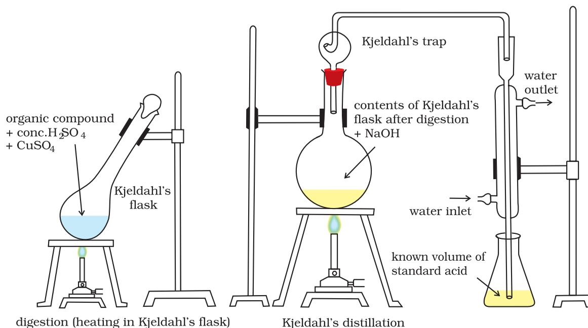
**Fig. 8.16** Kjeldahl method. Nitrogen-containing compound is treated with concentrated  $H_2SO_4$  to get ammonium sulphate which liberates ammonia on treating with  $NaOH$ ; ammonia is absorbed in known volume of standard acid.
