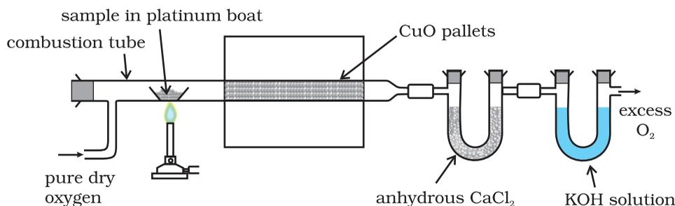
**Fig. 8.14** Estimation of carbon and hydrogen. Water and carbon dioxide formed on oxidation of substance are absorbed in anhydrous calcium chloride and potassium hydroxide solutions respectively contained in U tubes.
