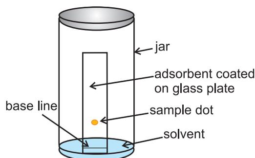
**Fig.8.12 (a)** Thin layer chromatography. Chromatogram being developed.
