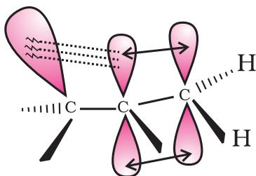
**Fig. 8.4(b)** Orbital diagram showing hyperconjugation in propene
