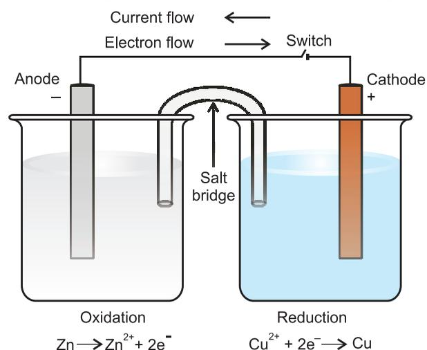
**Fig.7.3** The set-up for Daniell cell. Electrons produced at the anode due to oxidation of Zn travel through the external circuit to the cathode where these reduce the copper ions. The circuit is completed inside the cell by the migration of ions through the salt bridge. It may be noted that the direction of current is opposite to the direction of electron flow.
