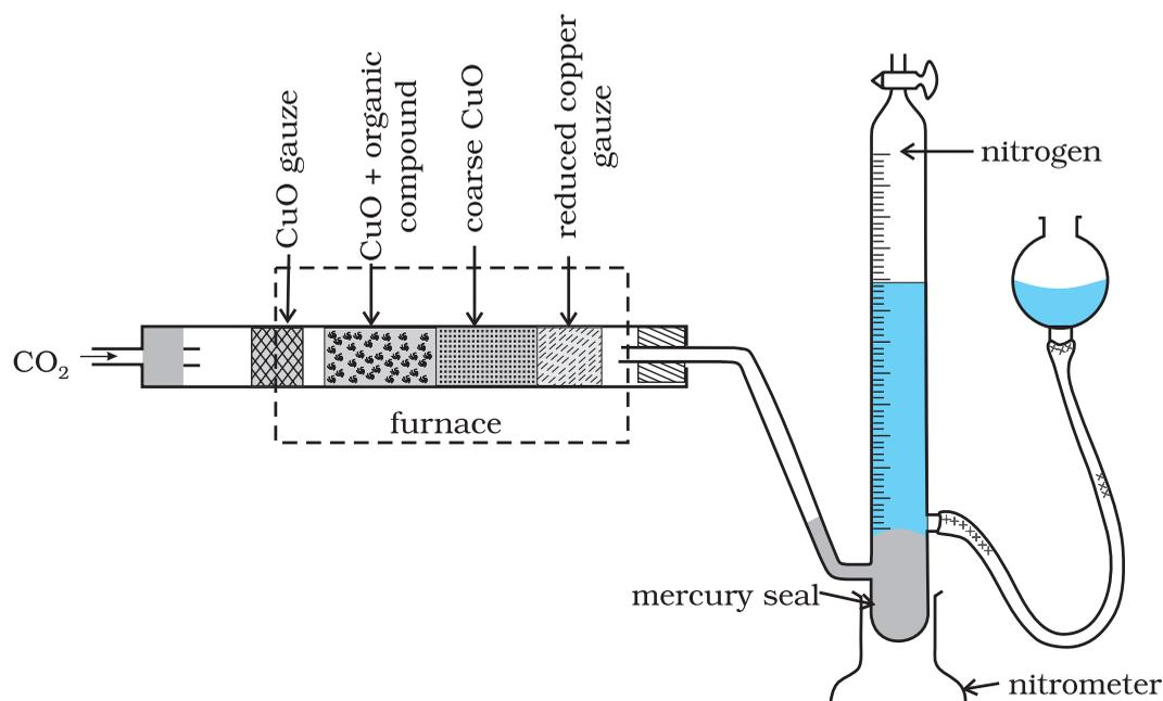
**Fig. 8.15** Dumas method. The organic compound yields nitrogen gas on heating it with copper(II) oxide in the presence of  $\text{CO}_2$  gas. The mixture of gases is collected over potassium hydroxide solution in which  $\text{CO}_2$  is absorbed and volume of nitrogen gas is determined.
